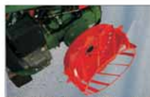
metal grid wheels, special CaneThumper attachment for operating on steep slopes
